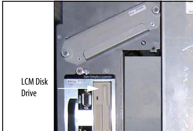
**Figure 1** *Insert Disk 1 in the LCM disk drive.*
