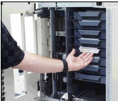
**Figure 3** Pull the old drive out of the drive slot.
