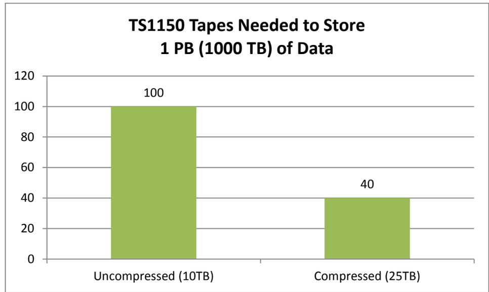
**Figure 5: TS1150 tapes needed to store 1 PB of data**
