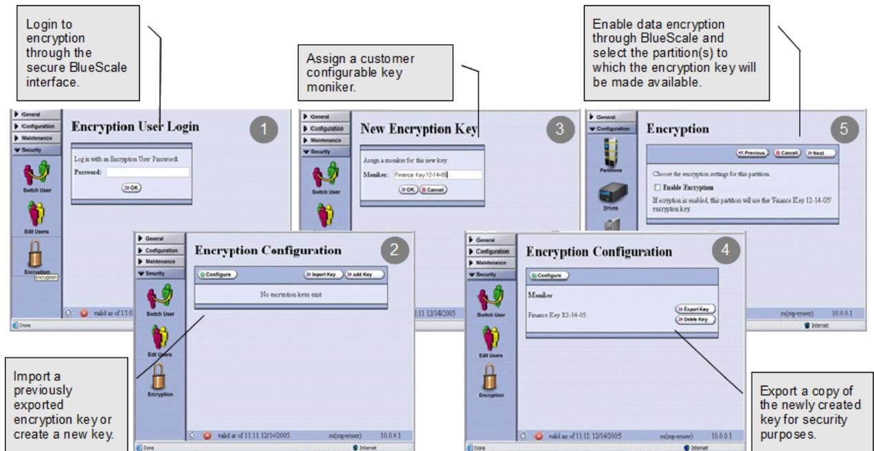
Figure 11: Encryption process in the BlueScale interface
