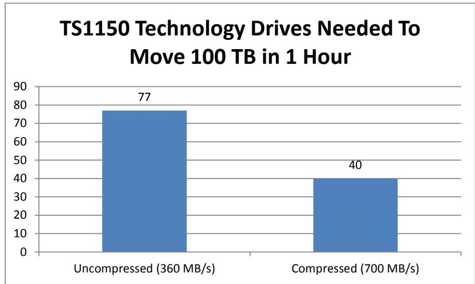
**Figure 6: TS1150 drives needed to move 100 TB in 1 hour**
