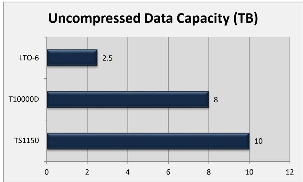
Figure 4: Uncompressed data capacity for major tape drive technologies
