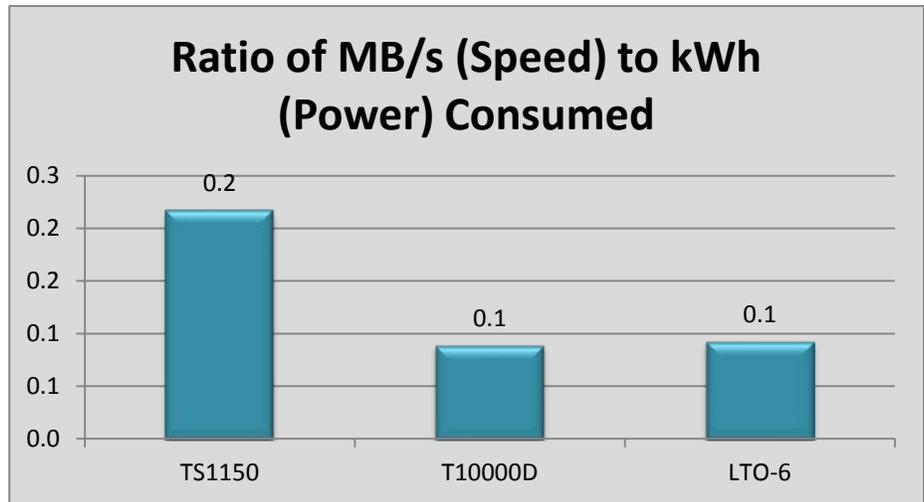
Figure 3: Ratio of speed to power consumed for major tape drive technologies
