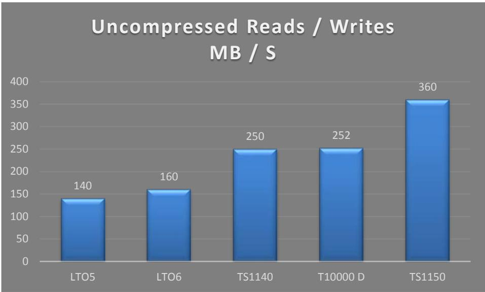
**Figure 1: Uncompressed reads and writes for major tape drive technologies**
