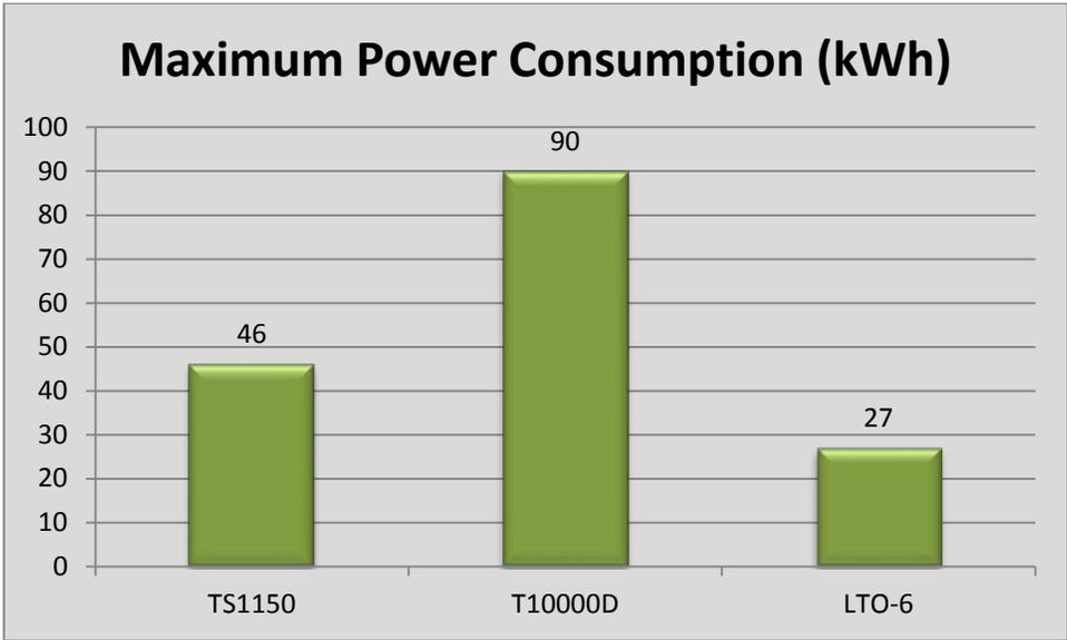
**Figure 2: Maximum power consumption for major tape drive technologies**
