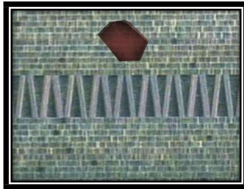
Figure 1: Tape media with a 100  $\mu\text{m}$  particle
