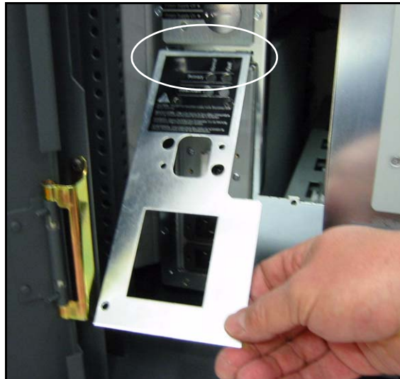
Figure 8 The faceplate tabs inserted in the chassis.
