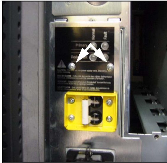
Figure 12 The two screws at the top of the faceplate.
