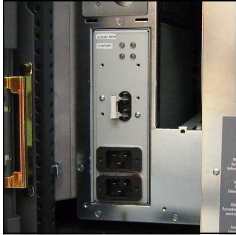
Figure 7 The dual AC module in the chassis.
